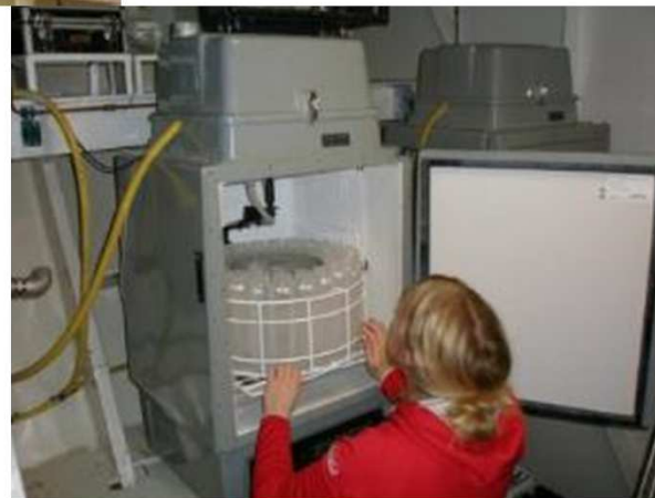
Automatic water sampling for total alkalinity, chlorophyll phytoplankton, salinity and CDOM.
