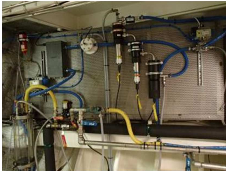
Salinity, temperature, oxygen, chl. fluorescence, turbidity, phycocyanin fluorescence and CDOM fluorescence
